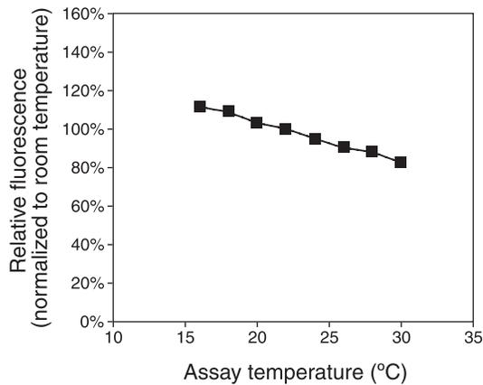
Figure 2. Plot of fluorescence vs. temperature for the Qubit<sup>®</sup> dsDNA HS Assay. The Qubit<sup>®</sup> assays are designed to be performed at room temperature, as temperature fluctuations can influence the accuracy of the assay.
